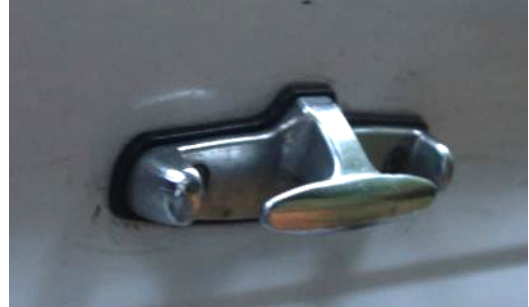
Well designed tie-down cleats. Anchor holes are separated 4" and use sturdy 5/16" bolts. Note these are shielded from the side which helps to avoid rope slip-off and reduces accidental catches on clothing.
