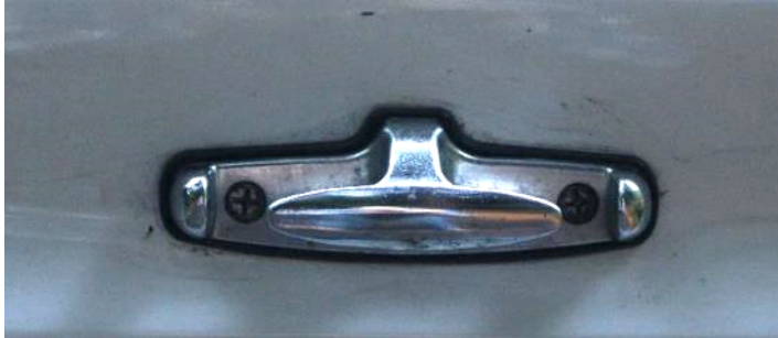
Well designed tie-down cleats. Anchor holes are separated 4" and use sturdy 5/16" bolts. Note these are shielded from the side which helps to avoid rope slip-off and reduces accidental catches on clothing.
