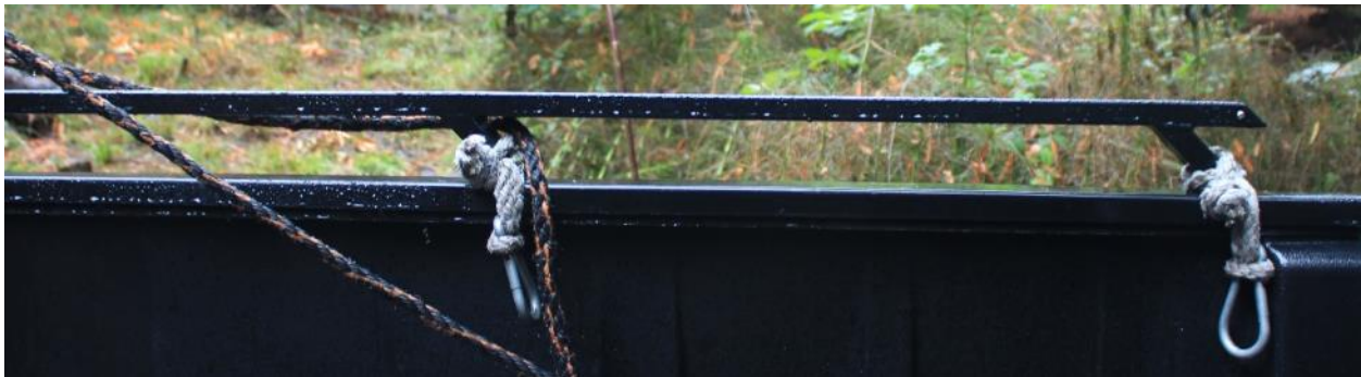
One of many designs for a rail. I added hefty loops with carabiner-style snap clips for convenience
